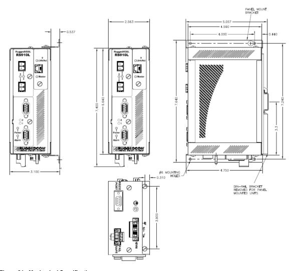
Figure 21 - Mechanical Specifications
